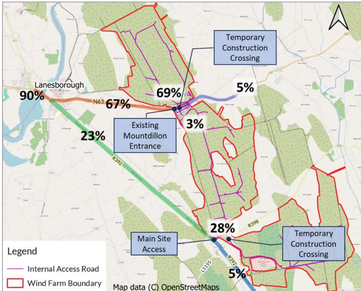
Figure 15-1: Construction Haul Route and Percentage HV Traffic Distribution
